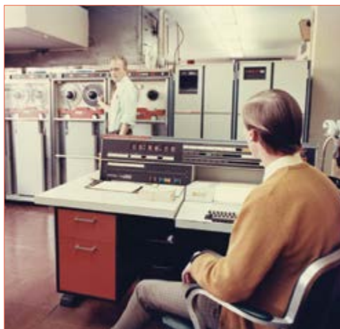
The UNIVAC 1108 computing system with the operator (Mr. Tillirson) at the control console and the assistant operator (Mr. Knight) mounting a data storage magnetic tape on one of the four tape units.
