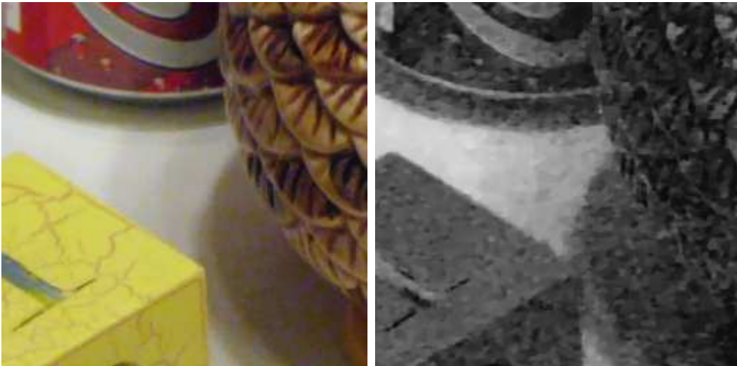
FIGURE 8. The denoised image by MTV in the RGB space (left) and its blue channel (right). Noticeable noise still exists due to high noise in blue channel even the recomposed image has most of the noise removed
